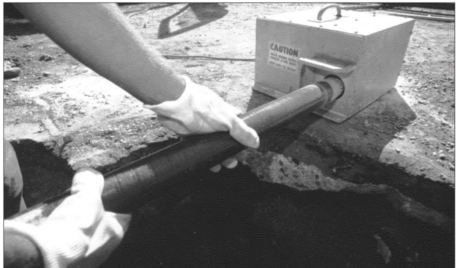
Fig. 5-4. Pipe in 2, 3 and 4-inch sizes is typically tapered using one of several powered tapering tools available from outside sources.
