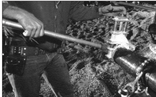
Fig. 5-3. Dualoy 3000/L can be tapered in all sizes using the Ameron Taper Maker. The ratchet handle makes Taper Maker convenient to use in confined spaces when repairing existing lines.
