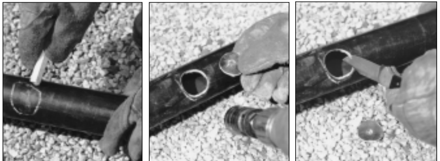
Fig. 1. Impact damage is generally apparent as a whitish discoloration.
